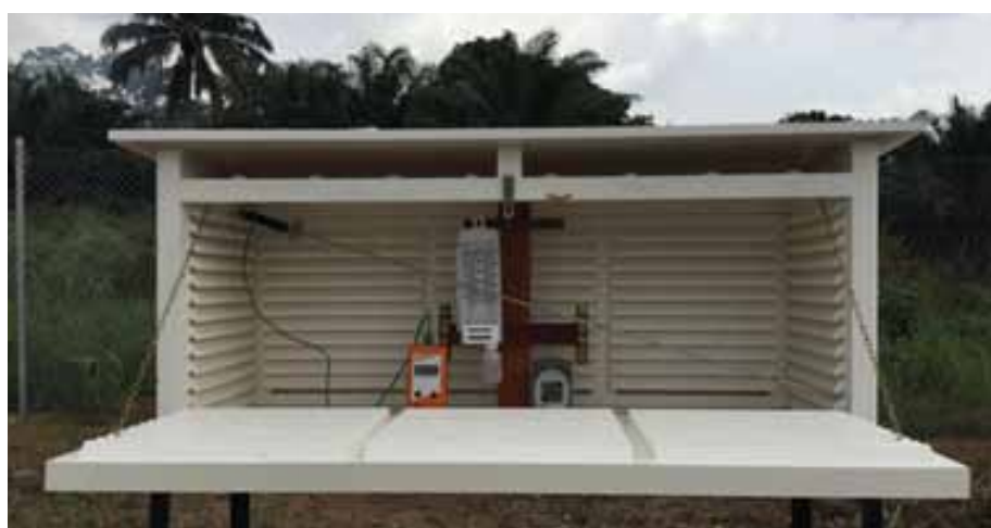
Ibu site: Stevenson Screen, Digital Soil Thermometer Wet/Dry Thermometer and Maximum/ Minimum Thermometer (NEWMAP)
