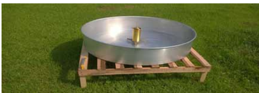
Bunya Dam Site: Evaporation Pan
